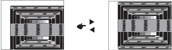
⑥ 1) Adjust the H Position so that the left side of the picture frame will move to the left edge of the display area.
