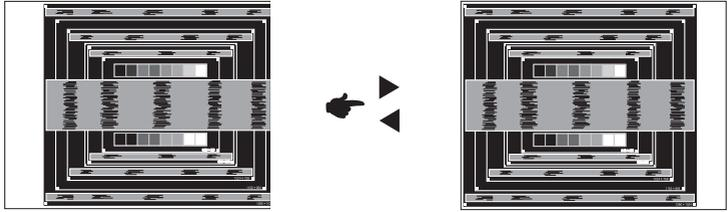
2) Stretch the right side of the picture frame to the right edge of the display area by adjusting the Clock.
