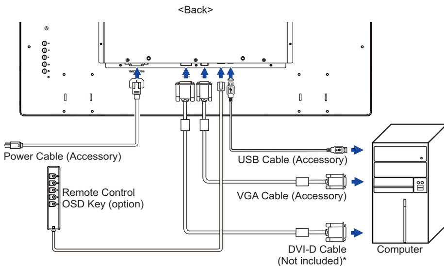
\* DVI-D cable is not supplied with the monitor. If you use low quality DVI-D cable, it may cause a result of electro-magnetic interference. Please contact the iiyama Support Centre in your country if you wish to connect the monitor via the DVI input.
