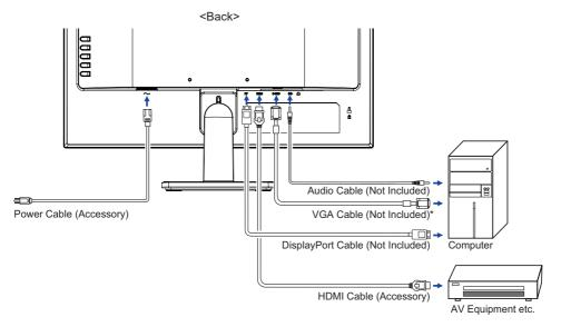
\* VGA cable is not supplied with the monitor. If you use low quality VGA cable, it may cause a result of electro-magnetic interference. Please contact the iiyama Support Centre in your country if you wish to connect the monitor via the VGA input. Signal Timing
